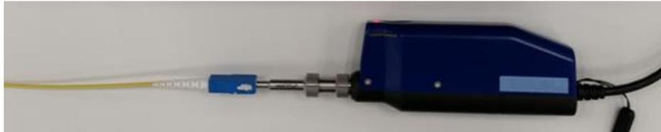
Tips are connected to the end of the VIP based on the shape of connector (adapter) to be connected.
